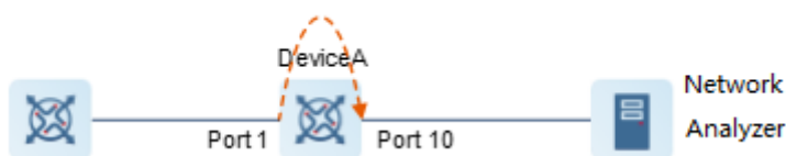
Figure 2-7 Operating Principle of Port Mirroring
